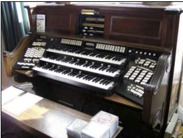
A working Aeolian Organ console at the private residence of Mr. Paul Morris, Exeter in Devon. The player roll is inserted above the trackerboard and taken up on a spindle beneath.
