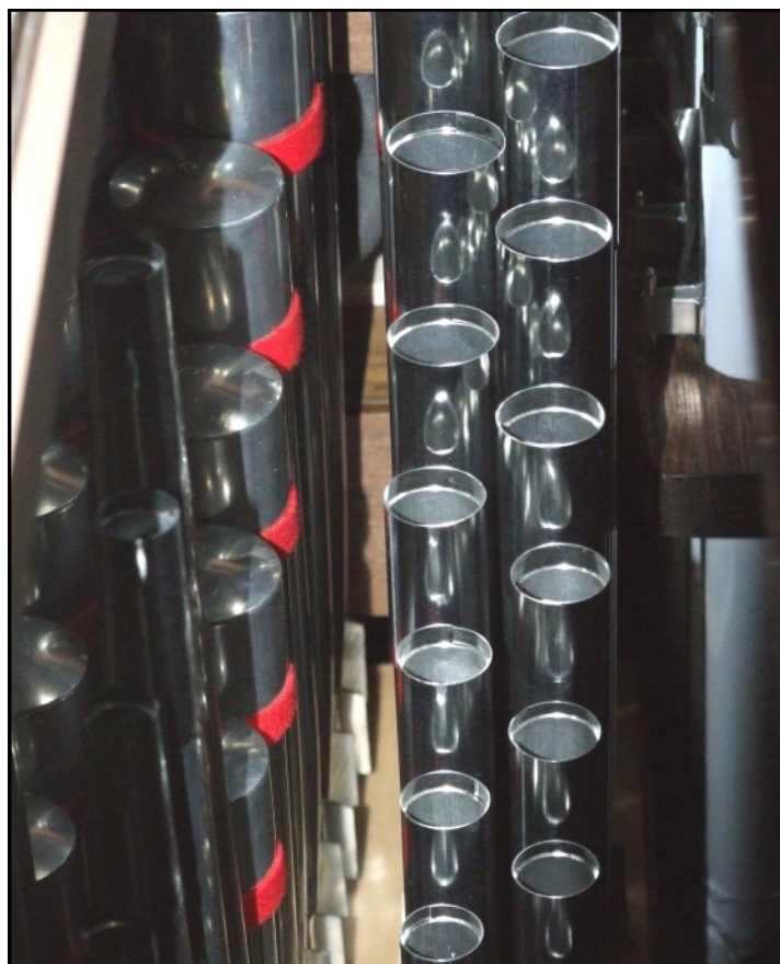
The compact interior of the Lincoln Cathedral continuo organ. Note the stopped flute with the red felt bands.
