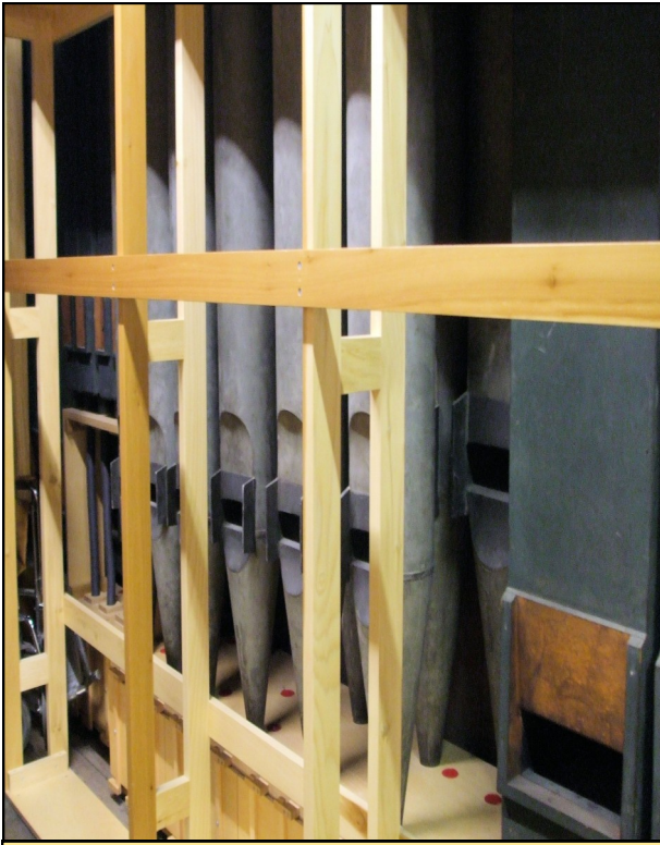
16' Bourdon and Diapason pipes at ground floor level in St. Paul's, Bedford.
